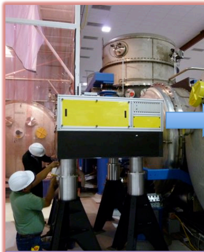
Squeezer table craned to its final location
